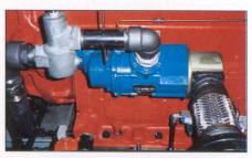
Pressure check ports on both starter inlet and exhaust allow easy troubleshooting of compressed starting air/gas supply valves, filters, piping and regulators. (Shown here TURBOTWIN Model T100-V and TURBOVALVE.)
