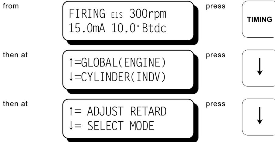
8.2 The first function can be used to save the current (temporary) individual offsets to EEPROM memory. When this is done, the ignition will load these new offset settings every time the engine starts.
