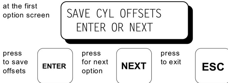
8.3 The NEXT mode function can be used to reset all cylinder timing offset values back to zero (both temporary memory and EEPROM memory).
