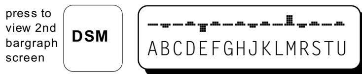
The third bargraph shows the relative magnitude of the Coefficient of Variation in voltage demand from cycle to cycle for each ignition output. The tallest vertical bars are the outputs with the greatest variation in voltage demand.
