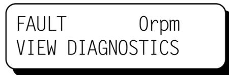
10.2 A warning represents the least severe classification of problems. The ignition will continue to fire in the presence of any warning. The list of warnings is expanded to include coil primary and secondary diagnostics when the Diagnostic Module is present. NOTE: These additional primary and secondary warnings do not operate the Fire Confirm Out Switch.
