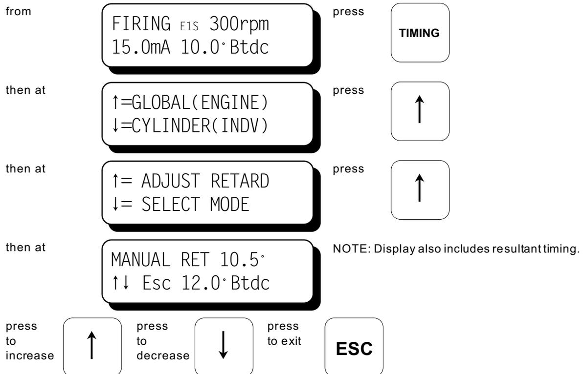
5.3 The increment of timing change is dependent on the number of holes or teeth being sensed. The minimum timing change is equal to "90/N" where N = no. of holes or teeth. EXAMPLE: For 360 holes, the minimum timing change increment is  $90/360 = 0.25$  degrees.
