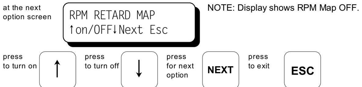
6.4 The Next mode selection can enable or disable the additional retard value controlled by the serial port. To use this option reference form CPU-2000 PI.
