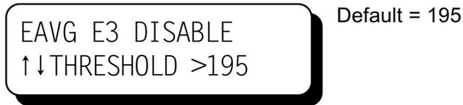
NOTE: Applications using firmware version 2.1 and a 32-output unit with memory engine cycle code "6" or "8" will use the larger of the two group average values ( 1AVG or 2AVG ) in place of EAVG when comparing to the energy thresholds.
