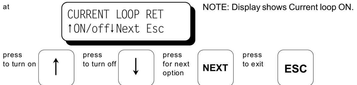
6.3 The Next mode selection can enable or disable the pre-configured retard curve controlled internally by engine RPM. To configure the RPM retard curve, reference form CPU-2000 PI.
