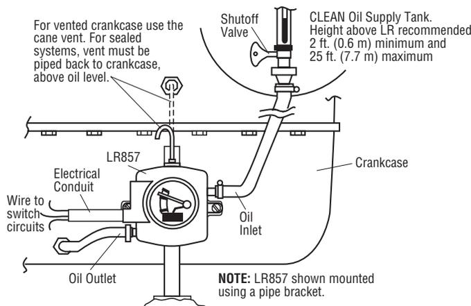
3. For sealed crankcases, connect a 1/4 in. (6 mm) O.D. tube from the crankcase to the tube fitting on the LR857 (see drawing below). For vented crankcases install the copper cane. **CAUTION:** The crankcase vent connection **MUST BE** above the oil level so that the tubing will not be restricted by oil splash, etc. Failure to install the tubing or cane vent will result in improper operation and oil spillage.
