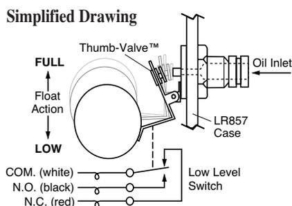
As the equipment uses oil, the float falls, providing immediate level compensation. At FULL position, the float holds the valve closed. If the clean oil supply is depleted and oil level continues to fall, the low level switch will operate an alarm or equipment shutdown.
