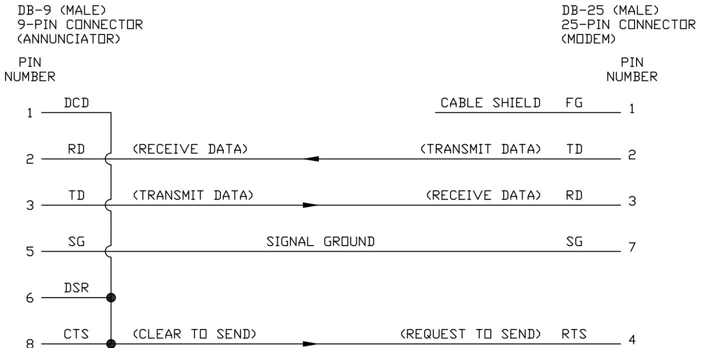
PINS NOT LISTED ARE NOT USED FOR THIS APPLICATION AND ARE LEFT OPEN.
