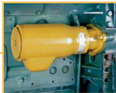
An ST650BP03R31 starter is shown mounted on a Detroit Diesel 12V-149R.
