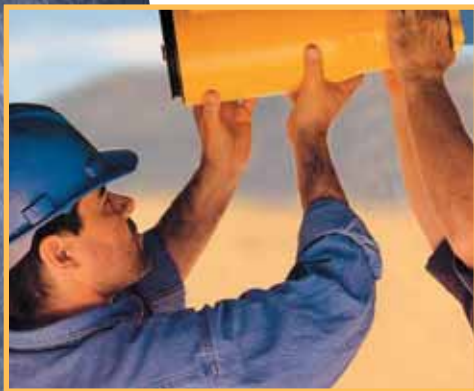
An ST650BP03R31 starter is shown being mounted on a CAT3512 used on a mine haul truck.
